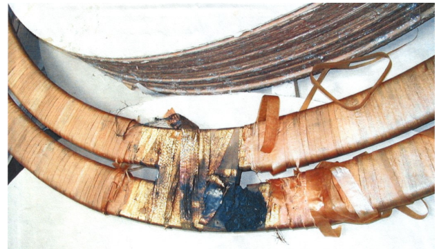
Fig. 6 Picture of the fault screen
